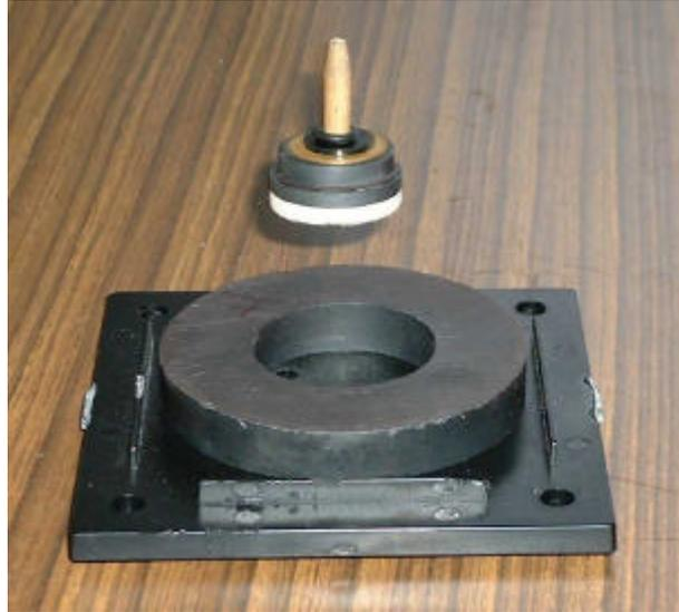
Fig. 1 Hand-made magnetically levitated spinning top on a base PM
