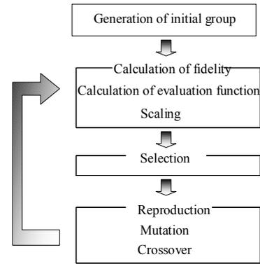
Figure 4 Procedure of the optimum value search by GA
