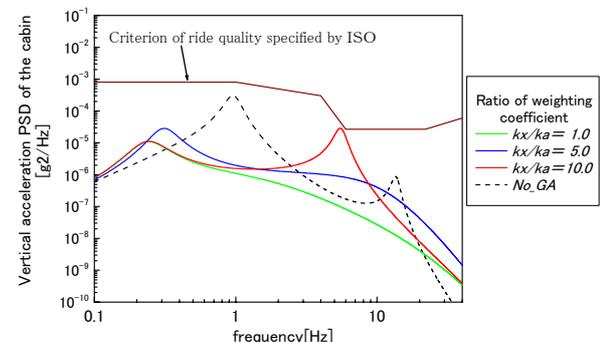
Figure 11 Frequency characteristics of vertical acceleration of the vehicle body
