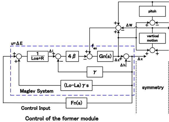
Figure 3 Block diagram of levitation model
