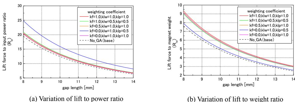
Figure 7 Static characteristics of the magnet
