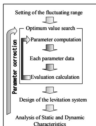
Figure 6 Flow of the whole simulation
