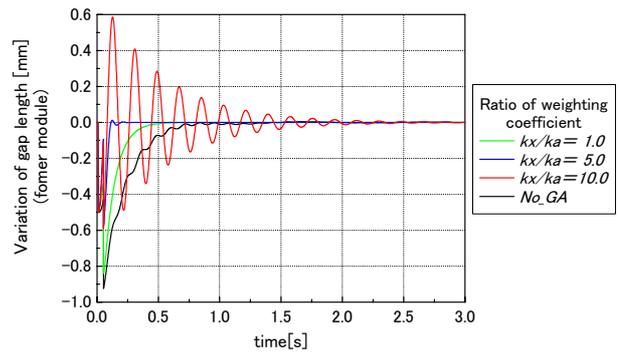
Figure 8 Step responses for the rail level difference ( $\Delta h=1[\text{mm}]$ )
