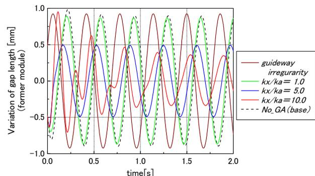
Figure 10 Gap length responses for the deflection of the track
