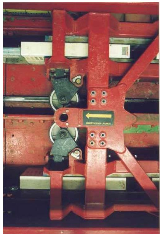
Figure 4 Magnet-stator-magnet sandwich on either side of pusher-car, vertical guide-rail in centre.
