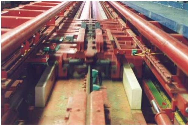
Figure 2 Accelerating pusher-car without train.
