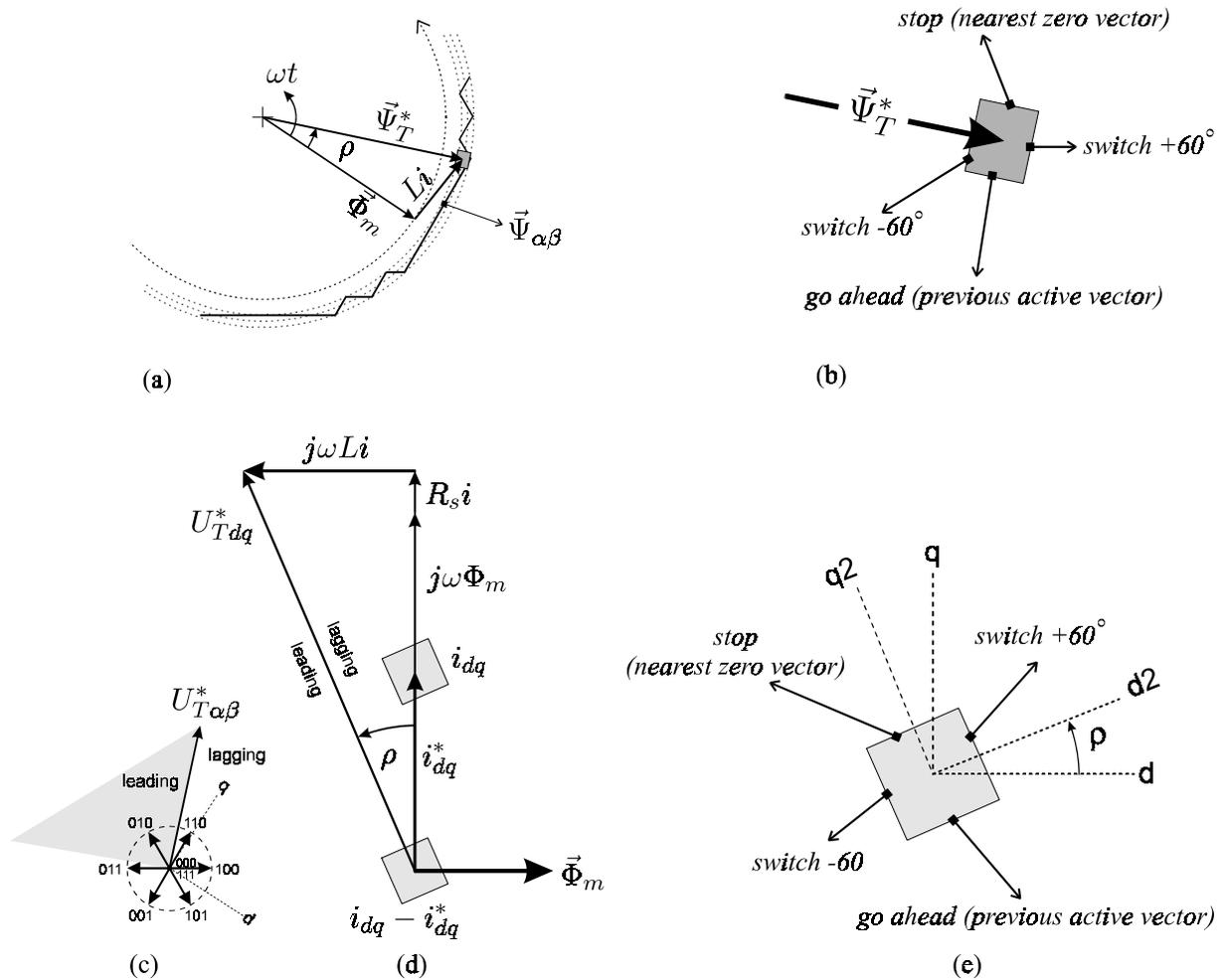
Figure 8 Asynchronous current control switching algorithm. (a) The switching box is aligned with the mean stator flux. (b) Switching actions on crossing boundaries when assuming a reference for terminal flux. (c) Definition of voltage vectors, mean terminal voltage vector and leading/lagging. (d) Vector representation of voltages and current in synchronous motor operating at load angle  $\rho$ . (e) Load angle correction of error box.
