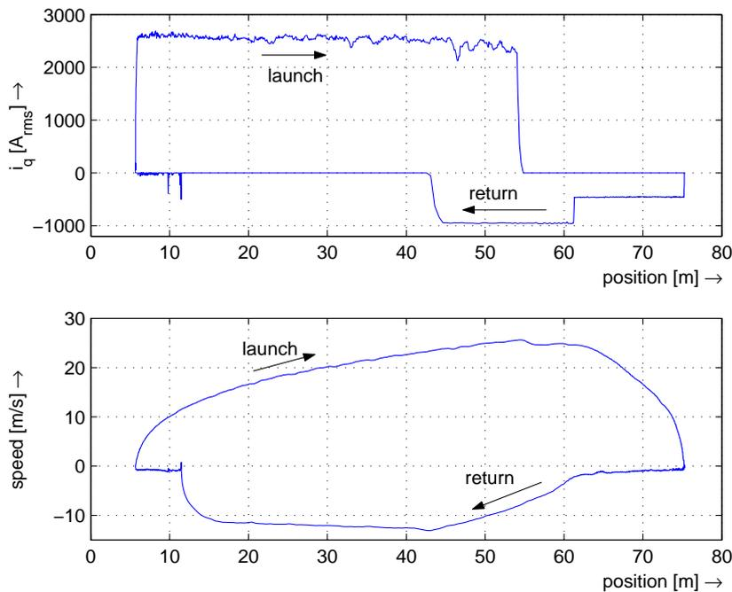
Figure 11 Current and pusher-car speed versus position during one cycle. Cycle consists of start, launch with train, brake without train, slow return through eddy current brakes and fast return to initial position.
