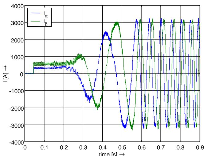
Figure 7 Measured data: start of launch with controlled build up to 2200A, sensor-less position.
