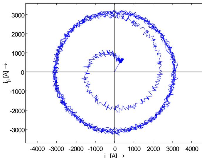
Figure 6 Measured data: current vector during launch in first second, sensor-less position estimation
