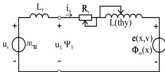
Figure 5 Simplified equivalent per phase circuit of LSM with switched stator.
