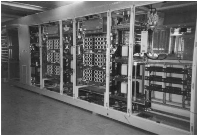
Figure 1 2.4MW inverter under construction
