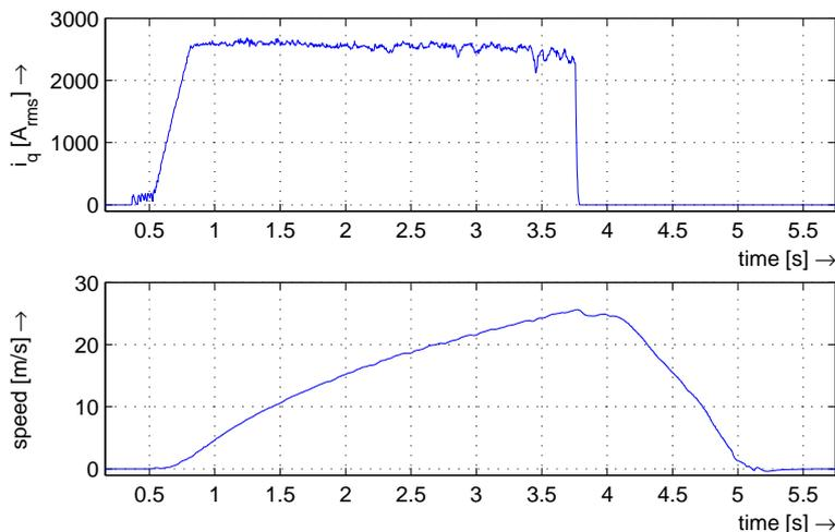
Figure 12 Launch with train to 25m/s. Current and speed versus time.
