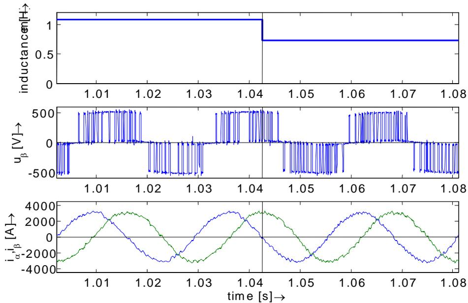
Figure 10 Measured data: stepwise change in inductance, switching frequency increases, current shape unaffected.
