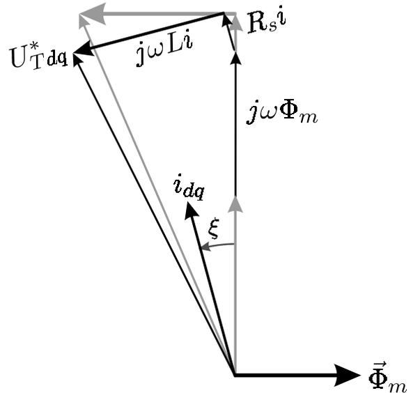
Figure 9 Introducing negative  $i_d$  to reduce required voltage.
