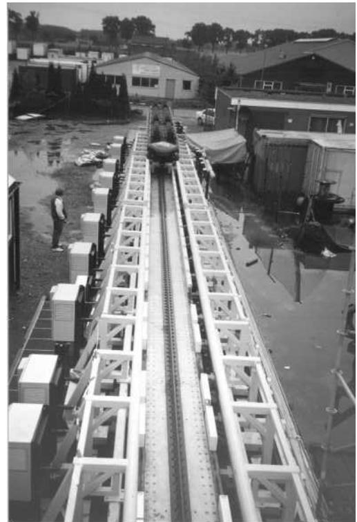
Figure 3 Test track of LSM, stators and guiding fin are visible. Pusher-car is underneath the train. Thyristors in boxes on left side.
