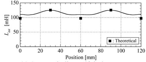
(a) Stator winding self-inductance.
