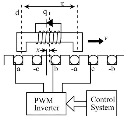
Fig. 1. Configuration of New LSM.
