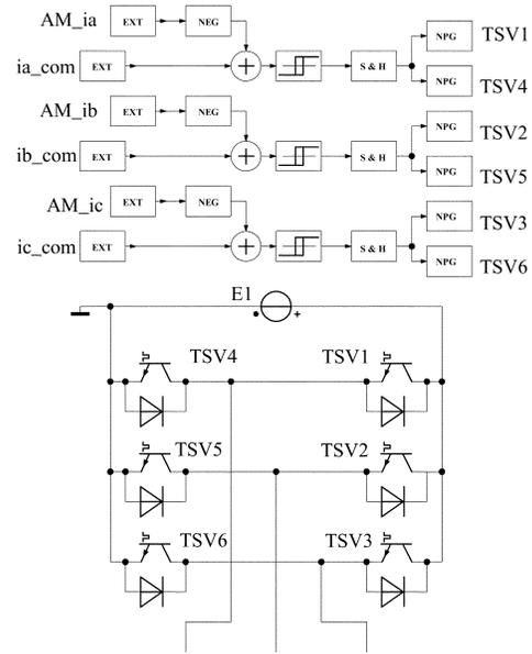
Fig. 9. Simulation Model of Control System.
