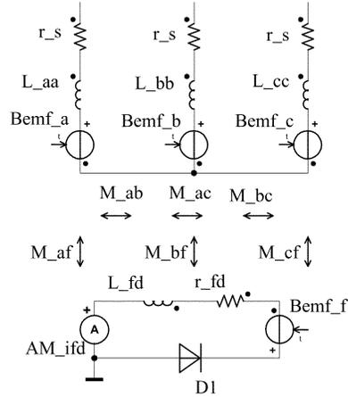
Fig. 8. Simulation Model of Experimental Motor.
