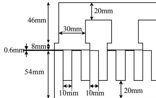
Fig. 4. Dimensions of Experimental Motor.
