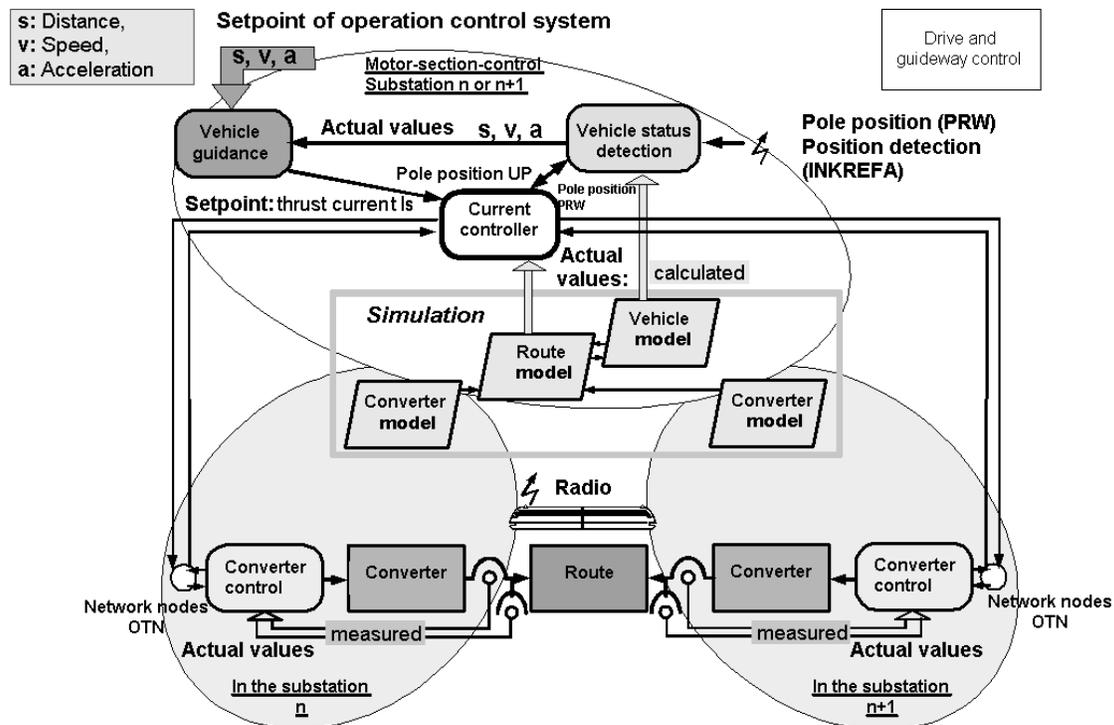
Fig. 3: Basic functional units of the TRANSRAPID drive control system and how they interact
