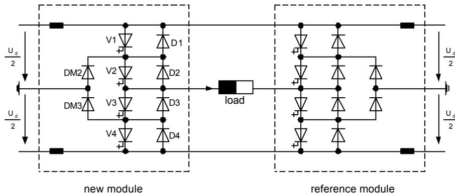
Fig. 8: Equivalent circuit during testing period
