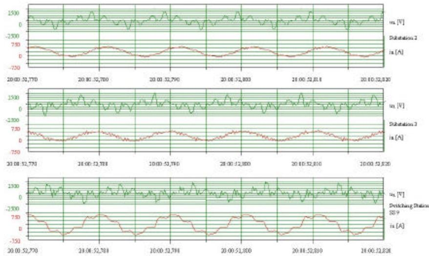
Fig. 6: Converter output voltage  $u_R$  and current  $i_R$  of substations UW 2 and UW 3 Stator section voltage  $u_{R\_SA}$  and current  $i_{R\_SA}$  (switch station SS9)
