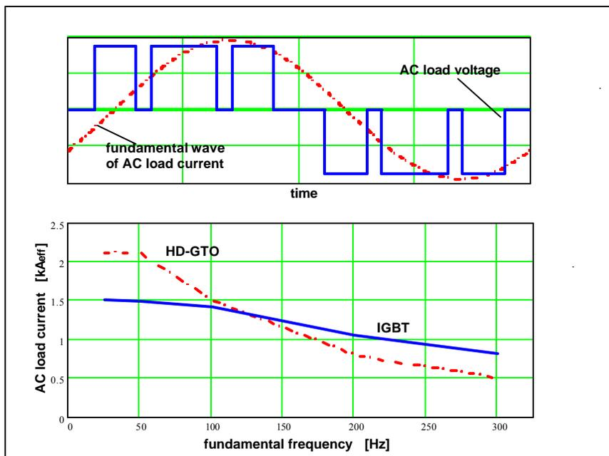
Fig. 13: Max. permissible AC rms-current of the module equipped with HD-GTO or PPI in dependence on fundamental frequency
