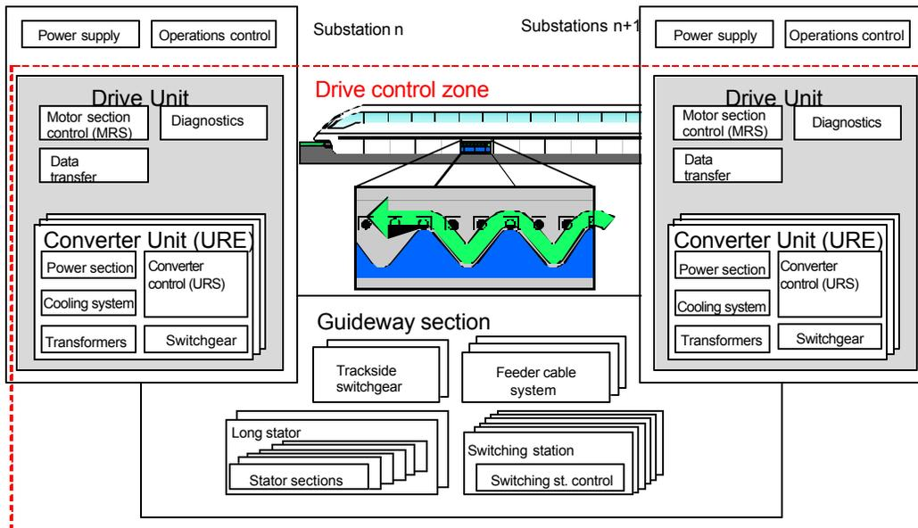
Fig. 1: Structure of the propulsion system
