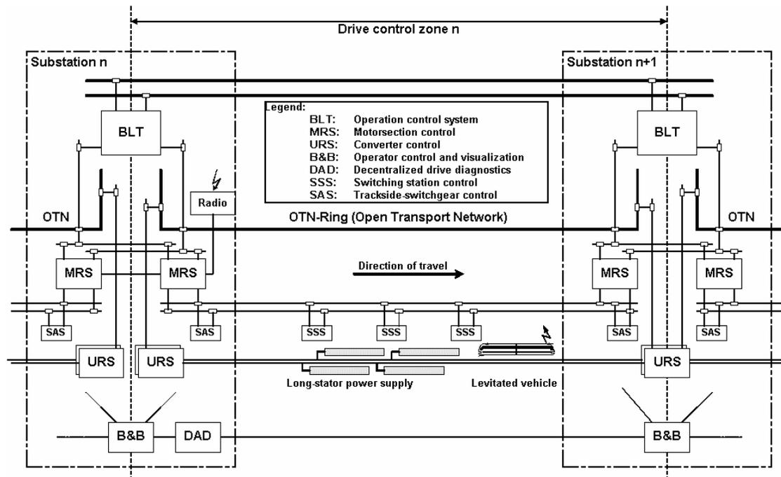
Fig. 2: Architecture of the TRANSRAPID drive control system
