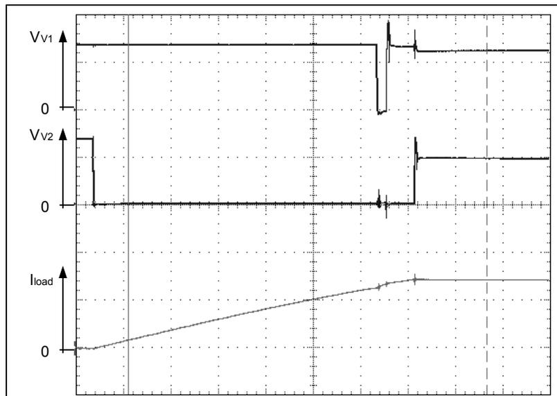
Fig. 10: Measurement of the switching capability (new module equipped with PPIs)
