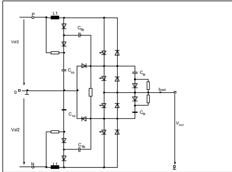
Fig. 7: Main circuit of the GTO-inverter phase including asymmetric snubber circuit
