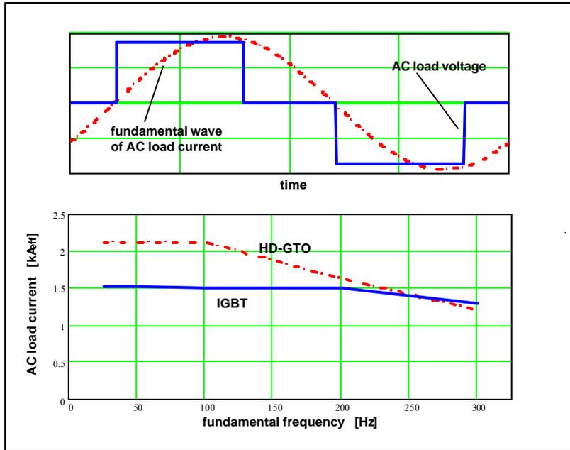
Fig. 12: Max. permissible AC rms-current of the module equipped with HD-GTO or PPI in dependence on fundamental frequency (assumption: pulse frequency according fundamental frequency)
