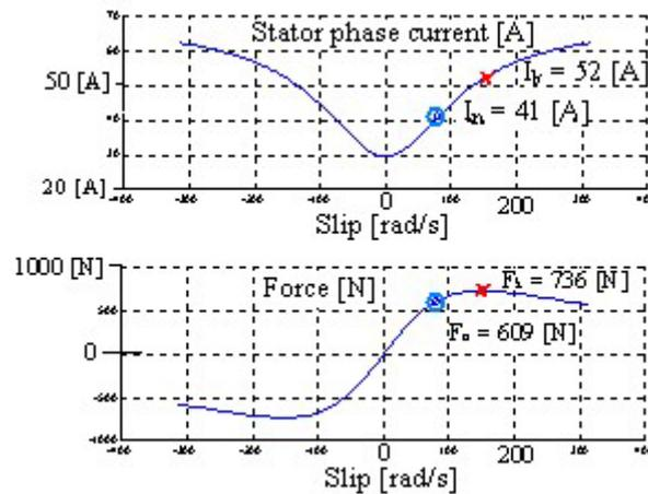
Figure 6 : Characteristic curves of the LIM
