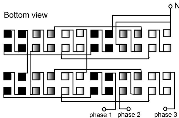
**Figure 2 : Windings of the LIM**
