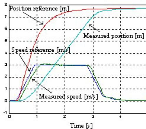
**Figure 10 : Speed and position regulation**
