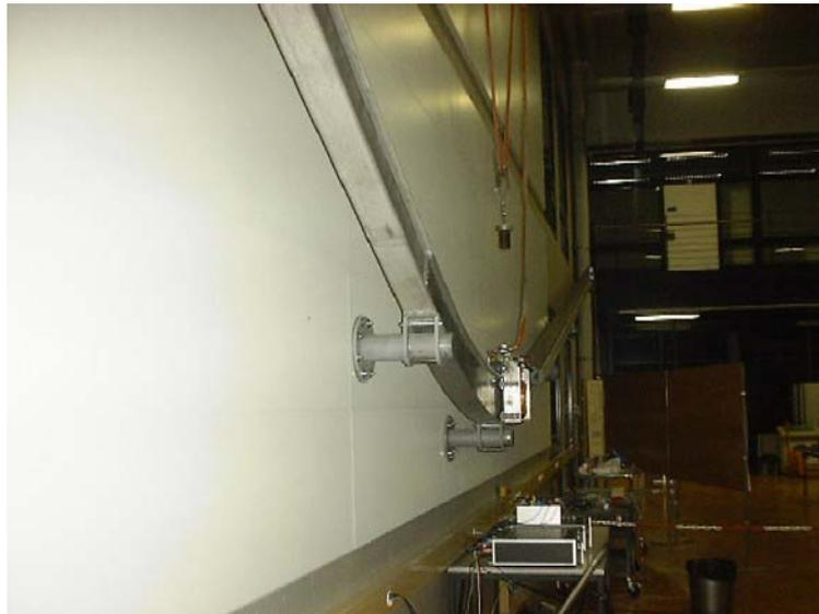
**Figure 3 : Rail of the LIM (rotor)**
