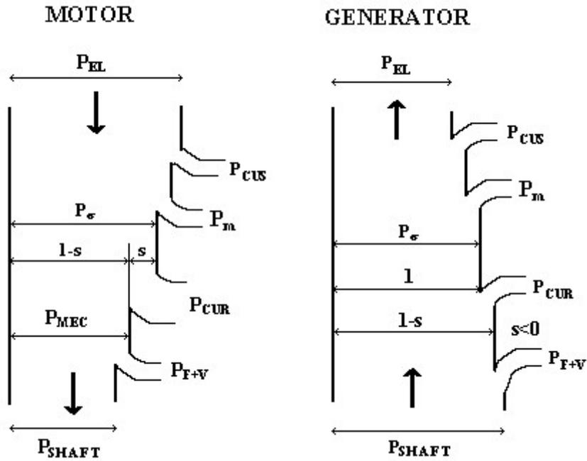
Figure 12 : Power flux in the motor
