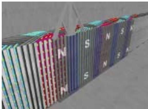
Figure 20: A single frame from an animation of the EMALS system showing one side of the stator only.
