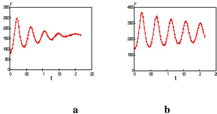
Fig.2. Typical time series of repulsive forces acting on moving magnet (current coil). Curves are figured out for  $V=60\text{m/s}$ . Curves a, b –for counter flux short-circuit contours with different lengths of magnet along direction of motion  $l=0.8\text{m}$  (a),  $l=1.2\text{m}$  (b).
