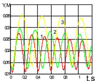
Fig.4 Time series of oscillations of moving current coil with different lengths.  $V=60$  m/s, 1- $l=0.8$  m, 2- $l=1.2$  m, 3- $l=1.4$  m.
