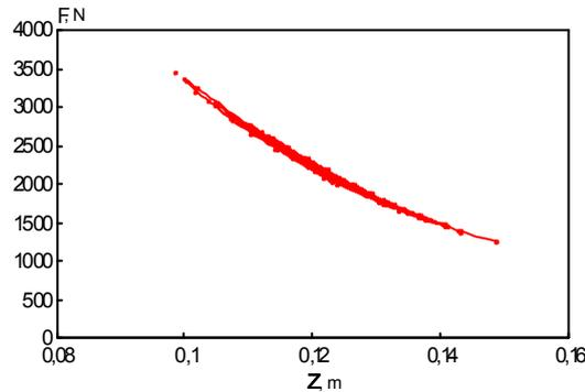
Fig.5 The dependence of repulsive force on distance between suspended current coil and short-circuiting contours arranged along direction of motion carried out in time series of dynamics evolved.
