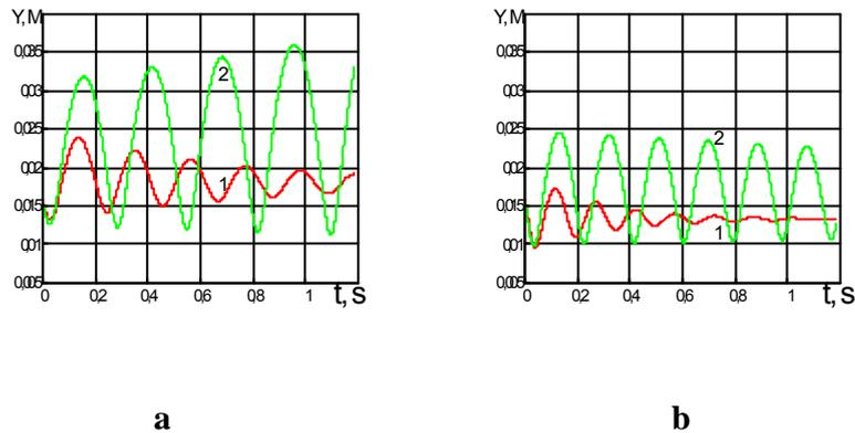
Fig.3 The time series of oscillations for different velocities of moving magnet and fixed lengths of short-circuit contours. Curve a -for  $l=0.8$  m,  $V=50$  m/s curve, b is for  $V=60$  m/s, 1-normal flux short-circuit contours, 2-counter flux short-circuit contours.
