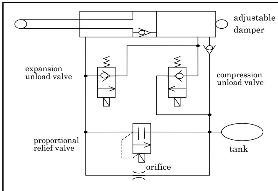
Fig. 2 Structure of an adjustable damper using a proportional relief valve system
