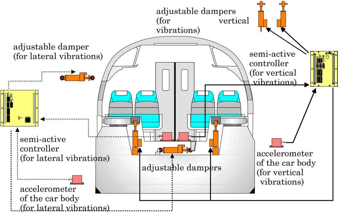
Fig. 1 Components of the semi-active suspension system
