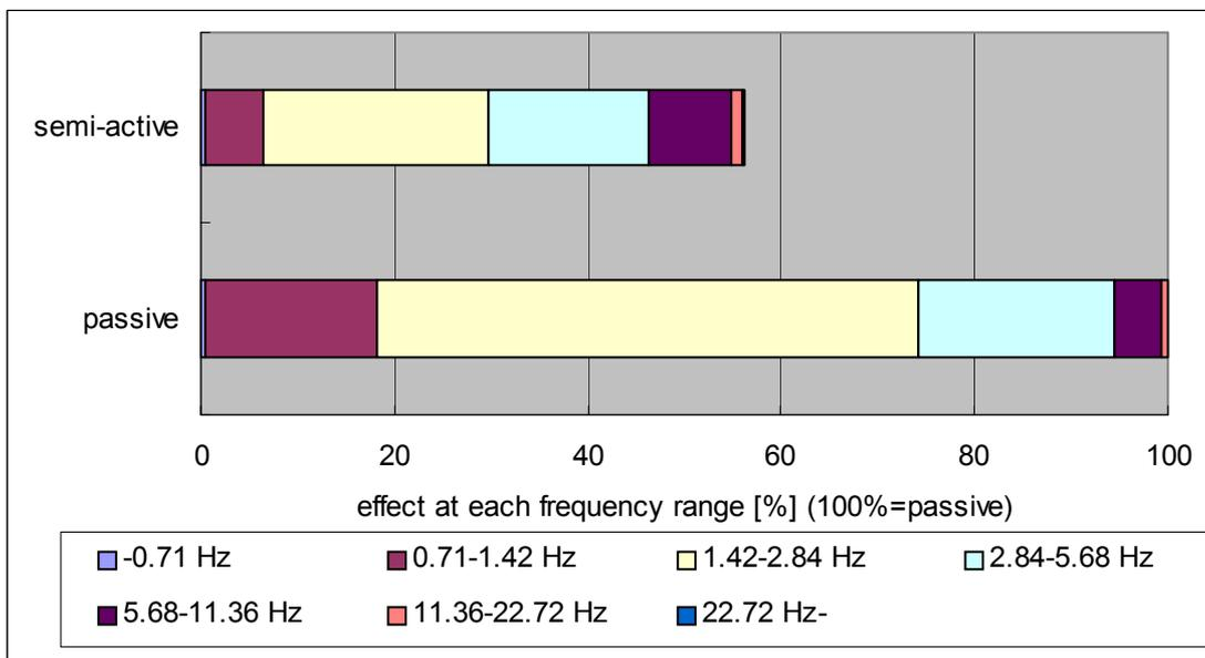
Fig. 5 Effect of lateral control at each frequency range
