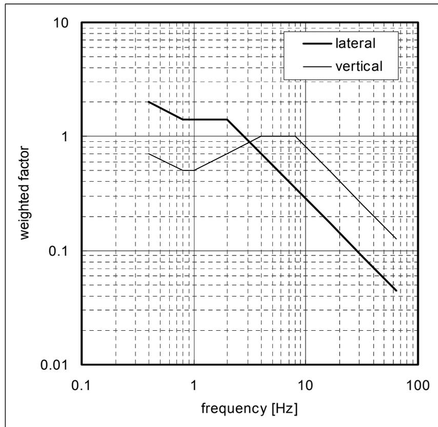
Fig. 3 Frequency weight curves for ride comfort
