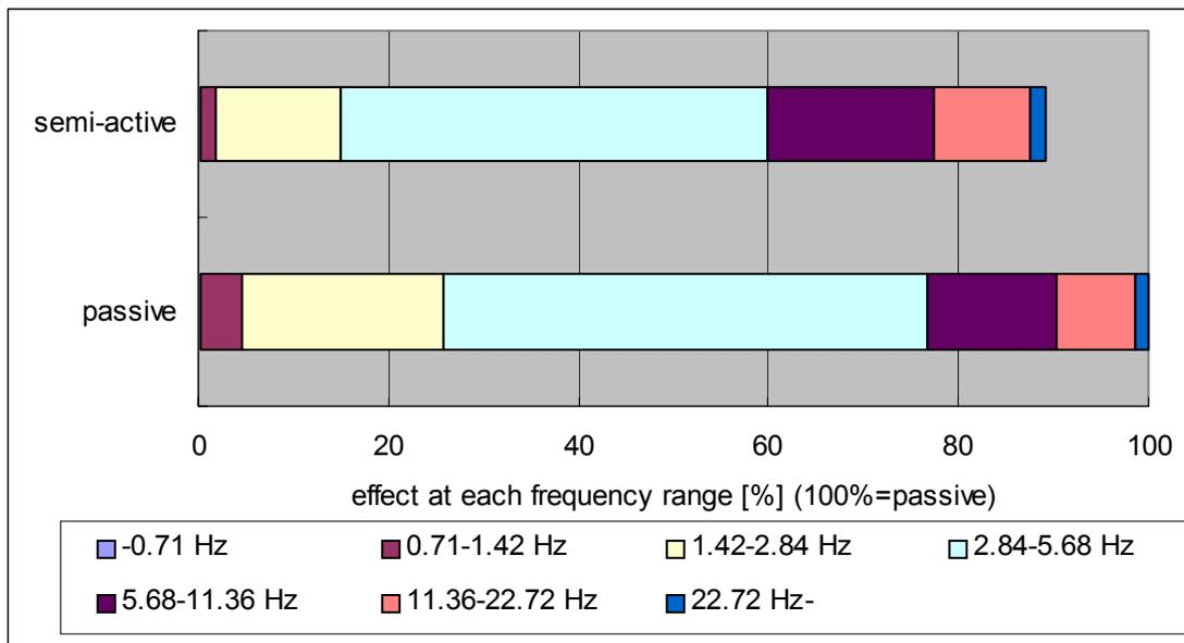
Fig. 7 Effect of vertical control at each frequency range
