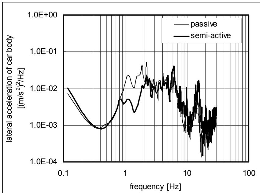
Fig. 4 PSD analysis of lateral accelerations of the car body
