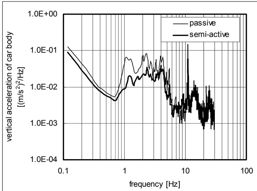
Fig. 6 PSD analysis of vertical accelerations of the car body
