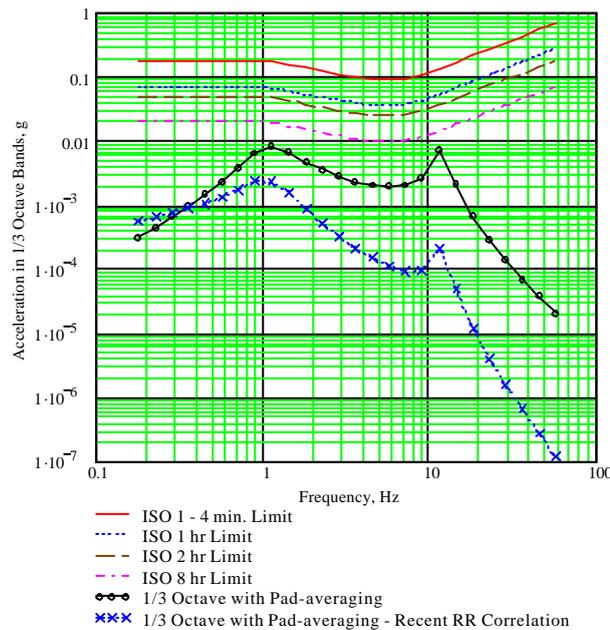
Figure 2. Dynamic Response in 1/3 Octave Bands of a Vehicle with Fifty Passengers. Analysis Used Two Roughness Models with Pad Averaging. Comparison is Made with ISO Standards.
