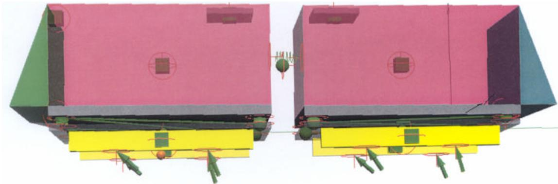
Figure 4. NASTRAN 6 dof model used in numerical simulation. The arrows at bottom are the magnetic forces applied to the model. An articulated joint connects the two halves of the vehicle. The model is accelerating right to left.
