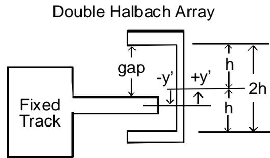
Figure 3. Definitions of magnetic geometry
