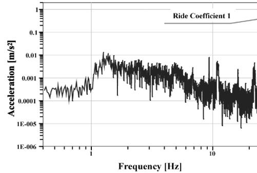
**Fig. 12 Horizontal Acceleration Spectrum**
