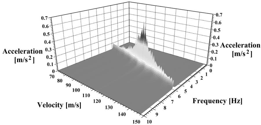
**Fig. 8 Vertical acceleration spectrum of the middle cabin**
