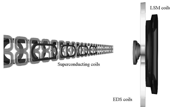
**Fig. 5 Image of the coil system**
