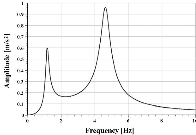
**Fig. 3 Vertical acceleration of car for one-dimensional analysis model**
