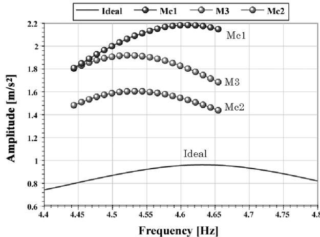
**Fig. 9 Vertical acceleration spectrum of the cabins (around 4.63 Hz)**
