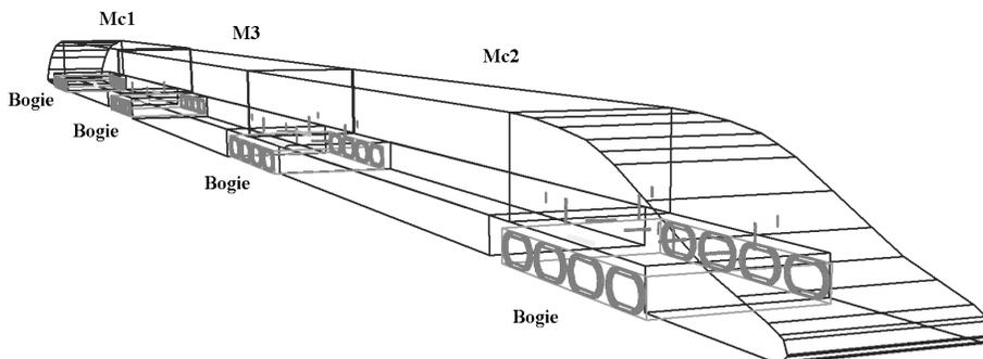
**Fig. 1 Wire frame of analysis model for the superconducting maglev vehicle in Japan**
