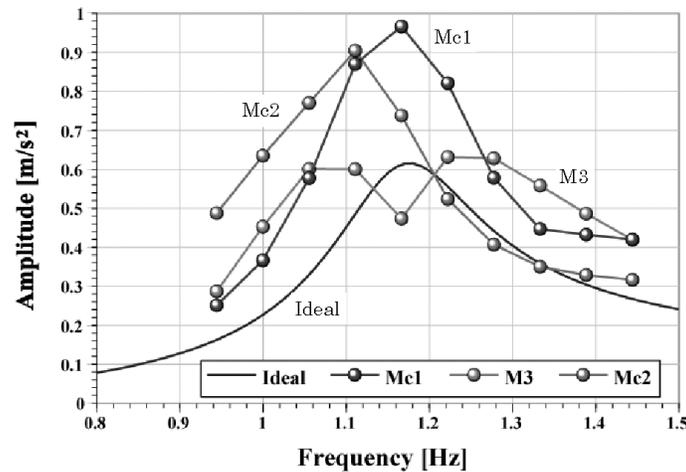
**Fig. 10** Vertical acceleration spectrum of the cabins (around 1.16 Hz)
