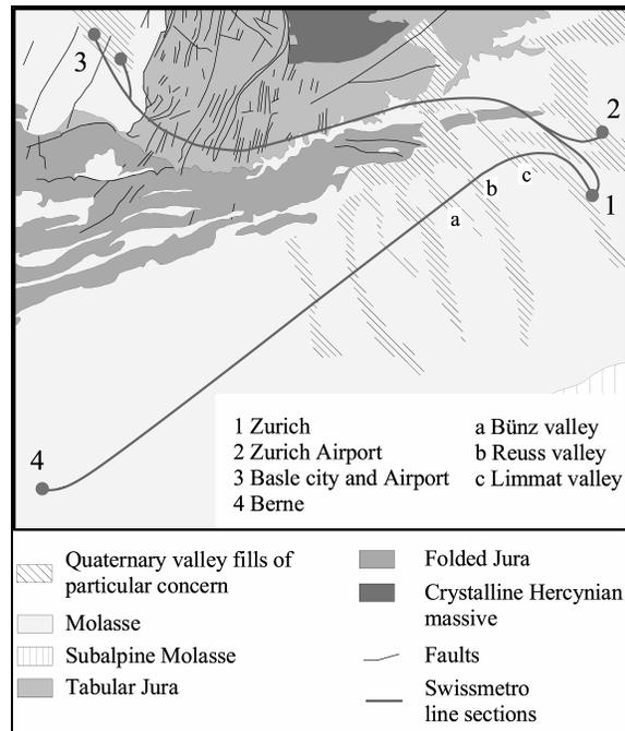
Figure 2. Tectonic map showing two segments of Swissmetro.
