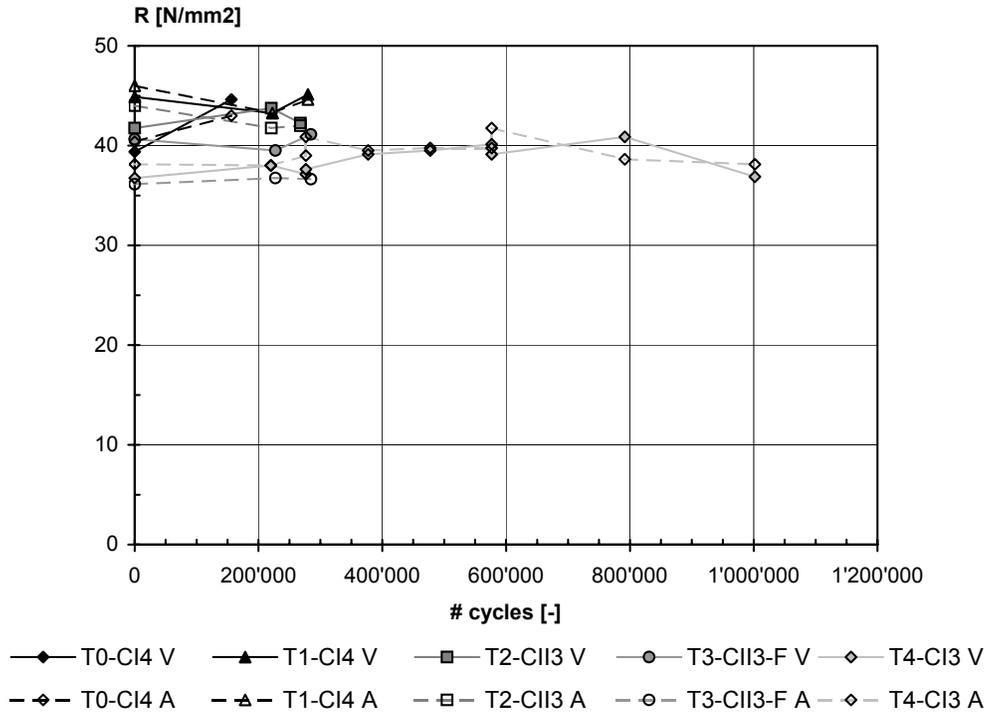
Figure 2: Surface concrete strength (Swiss hammer measurements)
