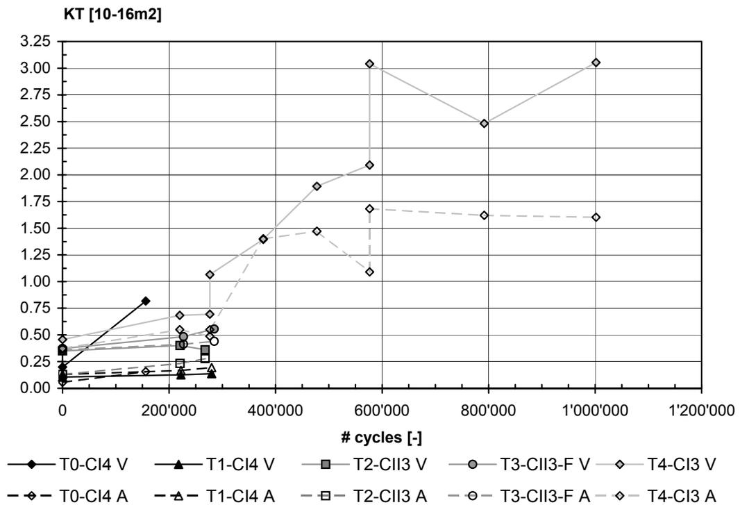
Figure 3: Air permeability measurements on the concrete surface (Torrent permeater)
