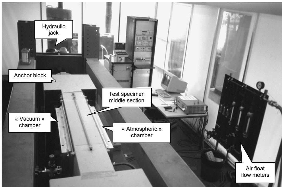
Figure 1: Test specimen T0 in the testing bench
