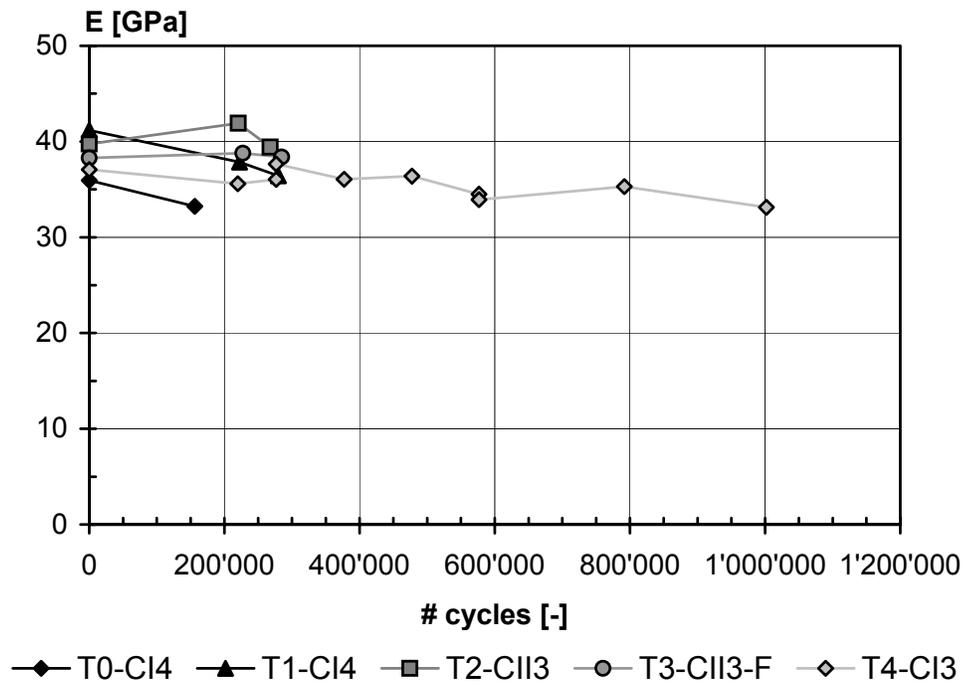
Figure 4: Ultrasound measurements of concrete modulus of elasticity (secant) for 5 specimens
