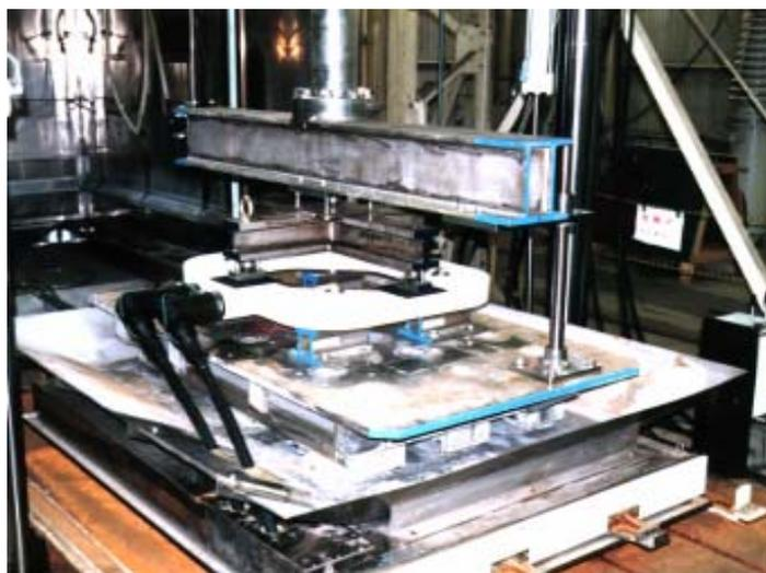
Fig. 5 Loading condition for the mechanical deterioration test
