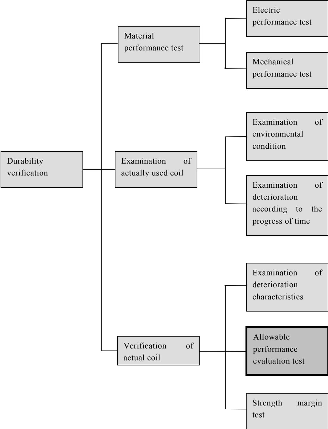
Fig. 1 Basic configuration of the durability verification test
