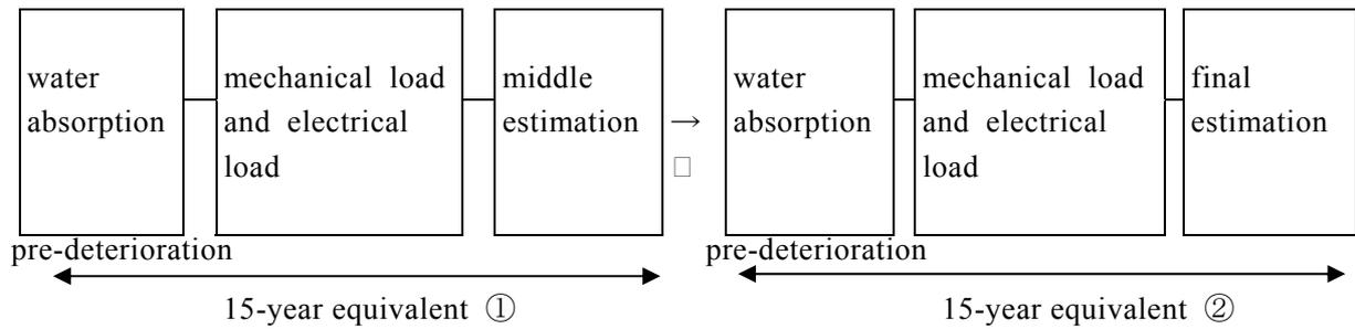
Fig. 4 Test configuration of the allowable performance evaluation
