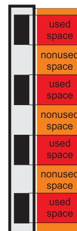
Figure 7: Many cabins in the same shaft increase the proportion of space.
