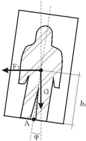
**Figure 14: Compensation of lateral forces by toppling the cabin**
