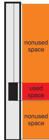
**Figure 1: Proportion of used space and occupied volume in today's elevator**
