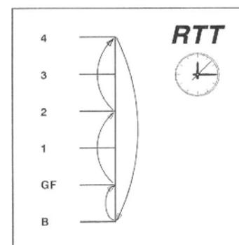
**Figure 4: Reducing the Round Trip Time increases the efficiency of a shaft.**
