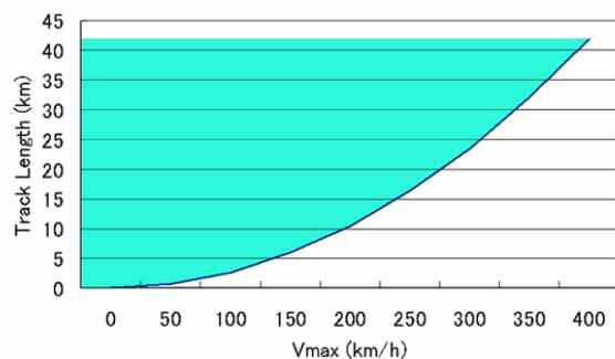
Fig.2 Length of Track needed to realize the schedule velocity more than 75% of the maximum operational velocity
