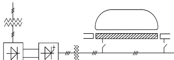
Fig. 5 Long-stator Drive System
