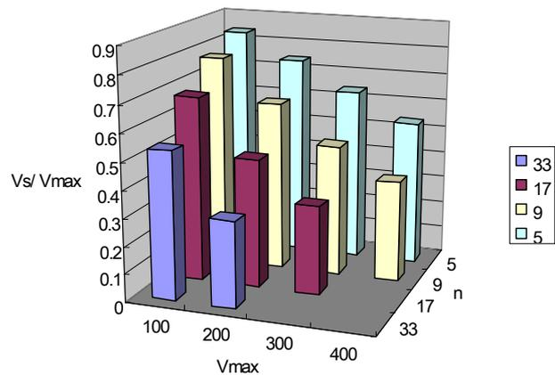
Fig.3 Ratio of Scheduled Velocity Vs against Maximum Operational Velocity Vmax with n Stops in Route
