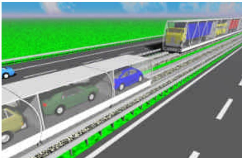
**Figure 1 : Autoshuttle at the centre of a motorway**
