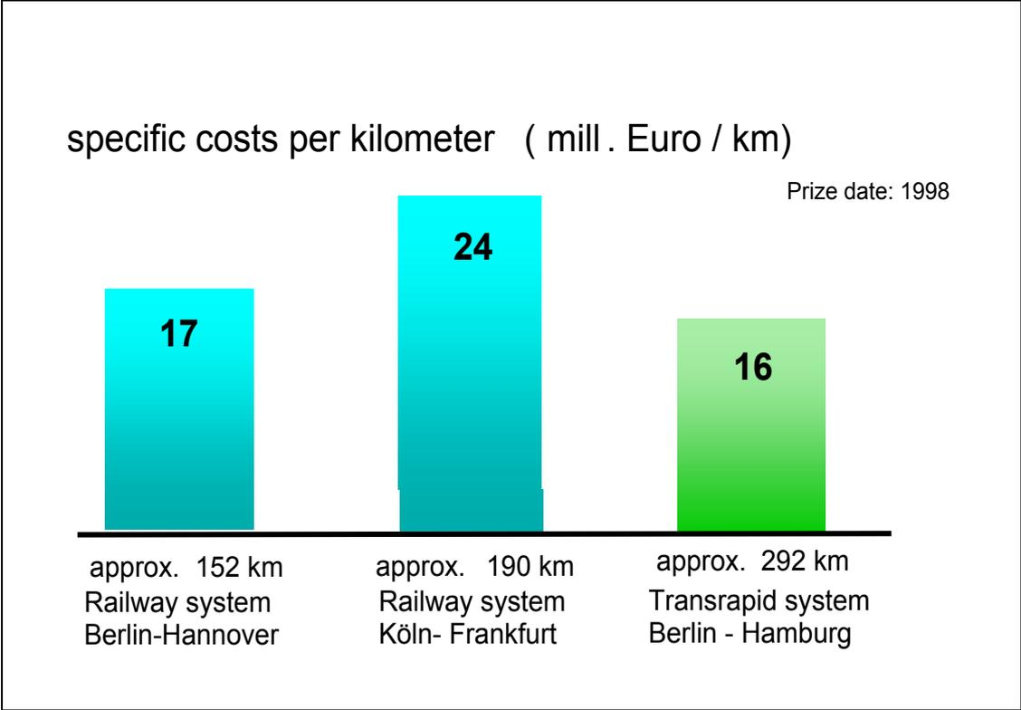
fig 2: guideway – investment Railway system and Transrapid system
