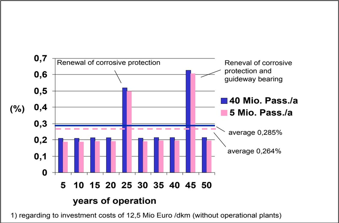
fig 3: Transrapid - guideway specific maintenance costs 1)
