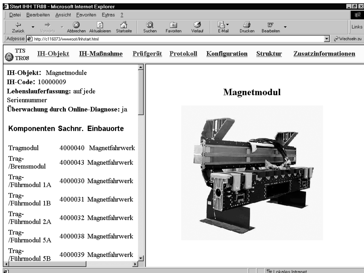
Figure 2: Detail from Hardware Object Description in Maintenance Manual
