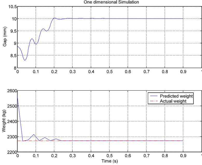
Figure 4 Gap position and weight estimate for a 30 ms update cycle.
