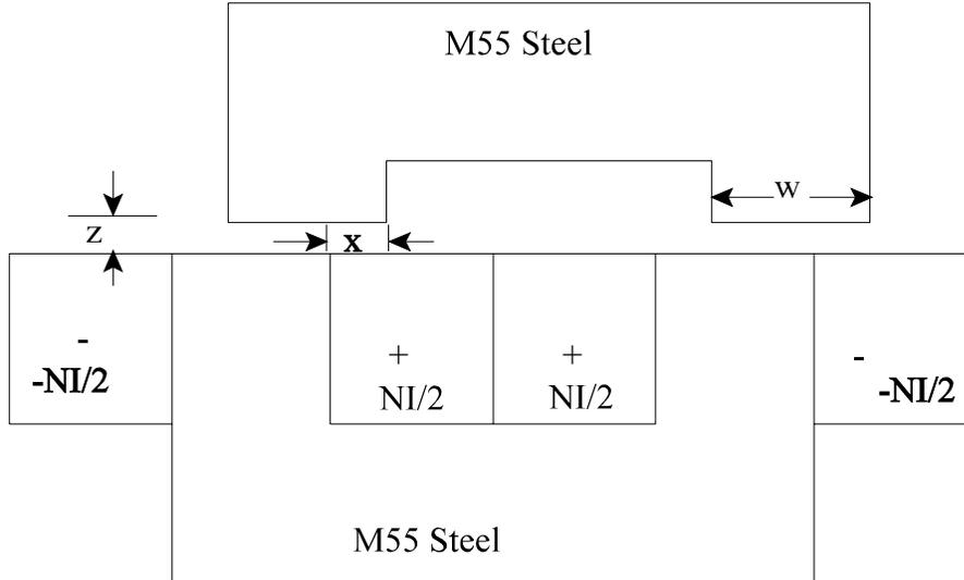
Figure 2 Displacement of the magnet yields natural restoring forces.
