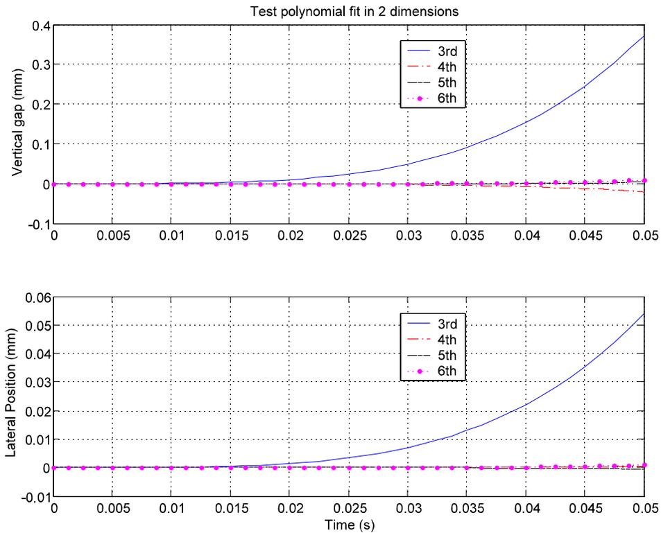
Figure 7 Comparison of bogie movement and polynomial prediction for 50 ms.
