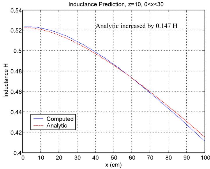
Figure 1 The analytic expression for inductance is quite good when leakage inductance is included.
