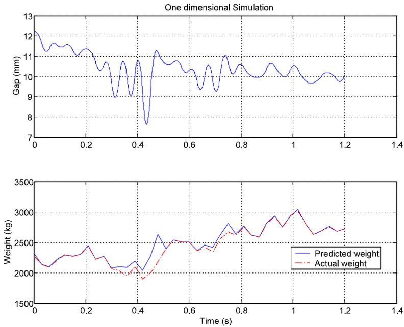
Figure 6 Response of the controller when the weight is randomly altered every 30 ms.
