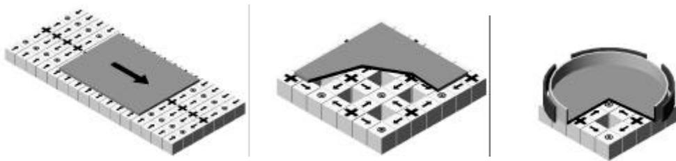
Fig. 6. a) Linear guide b) 6 DOF suspension c) Unstable contact-less suspension with active electrostatic actuators (acceleration sensing)
