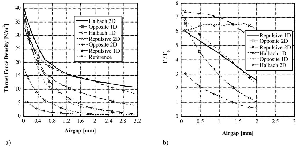
Fig. 3. a) Thrust force density for various NeFeB magnet arrangements for  $h = 5$  mm. b) Array performance  $F$ , compared to a monolithic reference  $F_0$ . The pyrolytic graphite specimen has a thickness of 1 mm.
