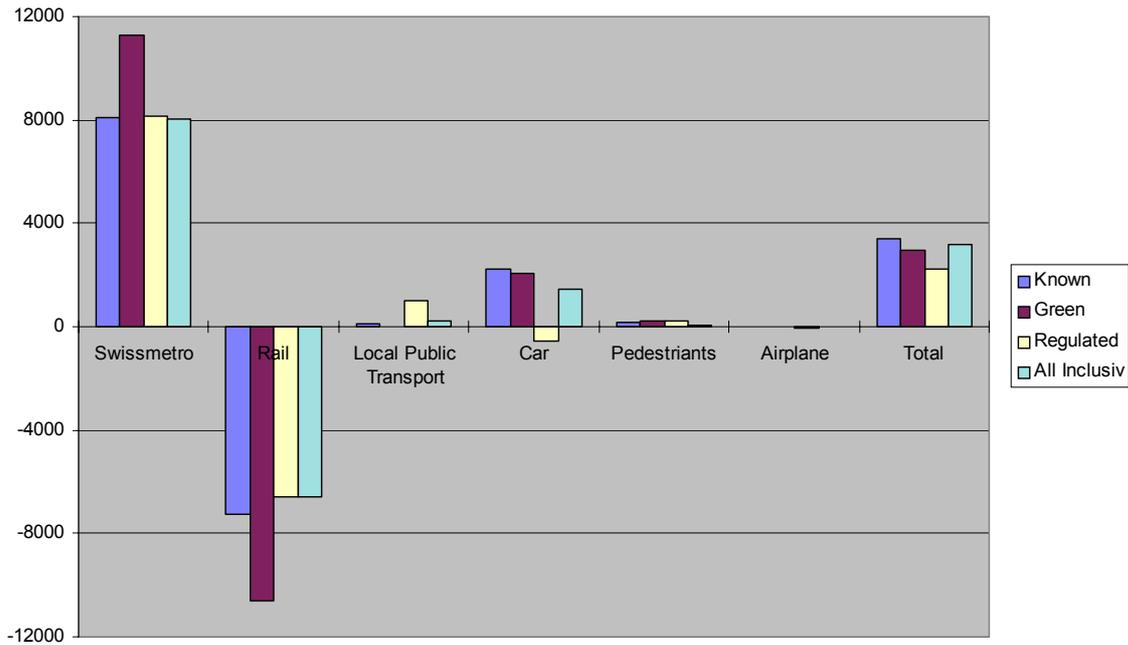
**Figure 5: Changes in the performance of different means of transportation (reference flows) in a comparison of the situations without and with Swissmetro; planning horizon is 2050; in millions of passenger kilometers in 2050**
