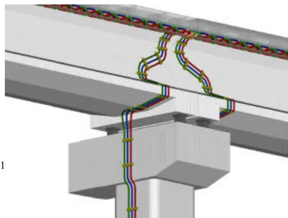
planning the global cable routing at the guideway constructions was planned on German side and were coordinated with the Chinese engineers as well as by means of local dates. The same one is valid for the arrangement of the motor windings within the stator packs. Also here very much detailed conditions were elaborated from German side concerning the project specifications of the Shanghai route.
