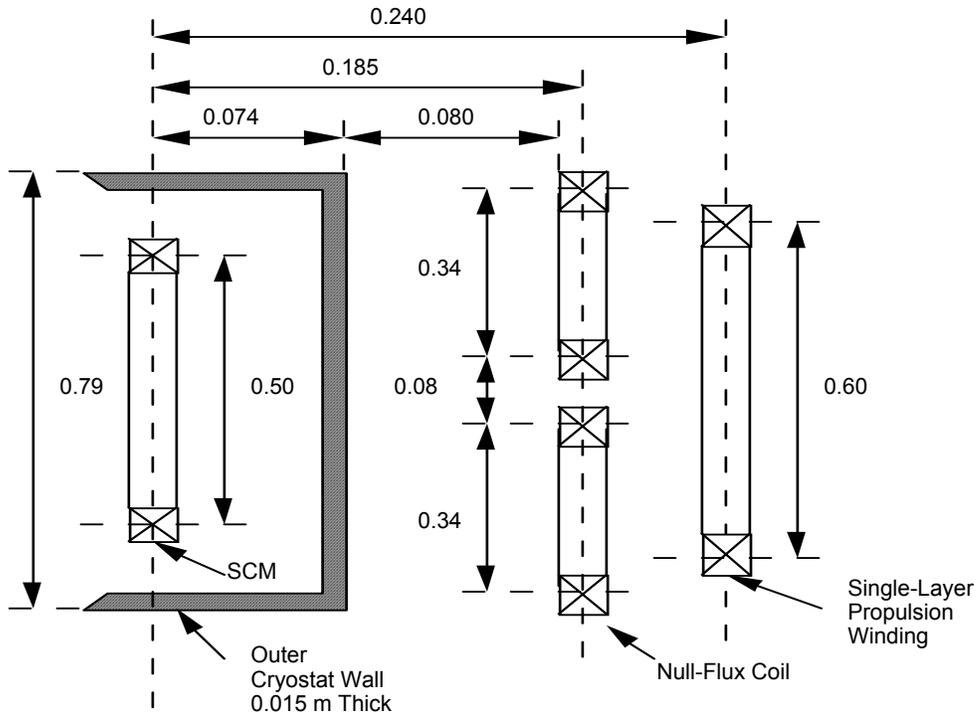
Figure 3. Shorted, Single-Turn Damping Coils Used to Simulate Damping Action of Damping Plate or Outer Cryostat Wall. For the Null-Flux Case An Upper and Lower Damping Coil is Used. For the Propulsion Coil Case a Single Damping Coil is Used.
