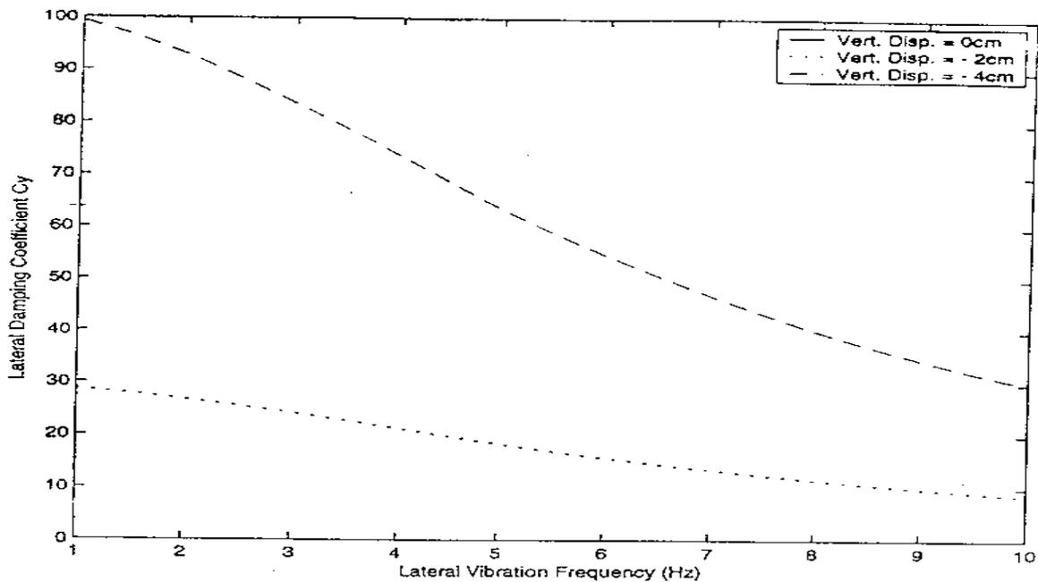
Figure 4b. Propulsion Coil – Damping Loop Lateral Damping Coefficient with Vertical Offset as a Parameter.
