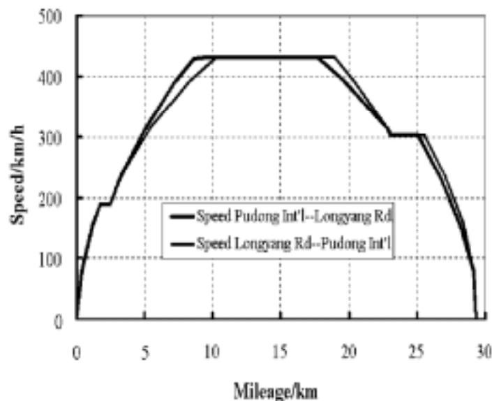
Fig. 4 Calculated Velocity Curves for Shanghai Line
